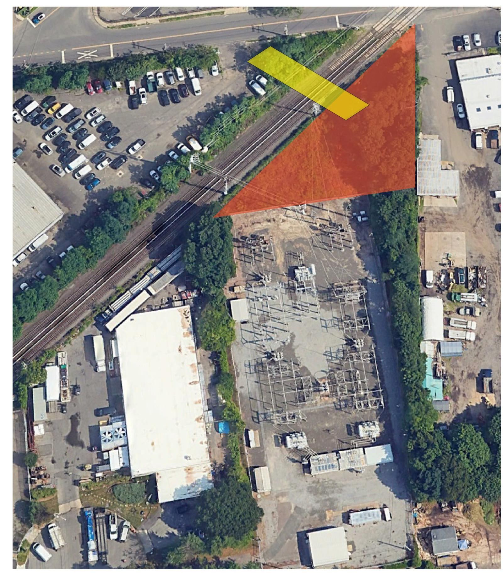
The existing Oakwood Substation will be expanded into the area in the orange triangle, including expansion of the fence line.
