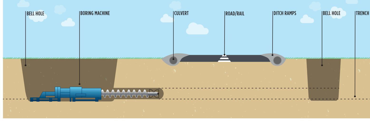
example of the trenchless crossing activity, commonly called auger bore installation.
